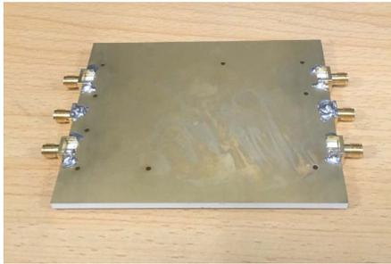
Fig. 19. Photograph of the fabricated Butler matrix prototype.
