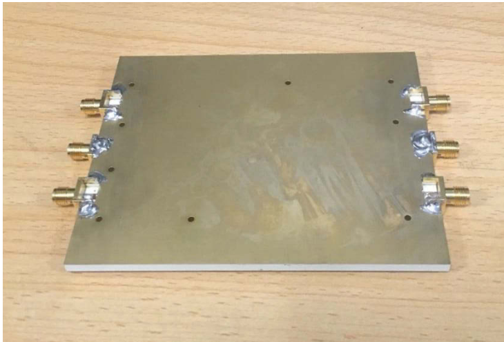
Figure 7.11 Photograph of the fabricated Butler matrix prototype.
