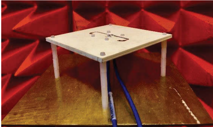
Figure 5.8 Prototype of the three-layer planarized dual-LP antenna.
